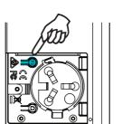
Press P2 on controller MOTOR RESPONSE
