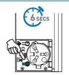
Repeat steps 1-6 for all motors. Once complete Press and hold the Lock button for 6 seconds while looking at the LED, and hold until solid.
