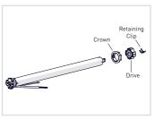
**Step 4.** Slide Motor into tube.
